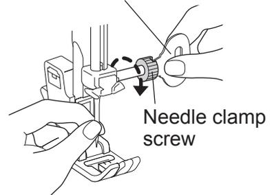
**3** Face the flat surface of the needle to the rear and insert until it makes contact with the pin.
