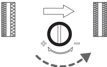
If the stitches are loose on the left side of the buttonhole, turn slightly in the “+” direction.
