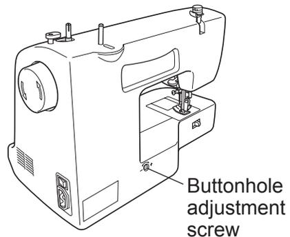
If the stitches are loose on the right side of the buttonhole, turn slightly in the “-” direction.
