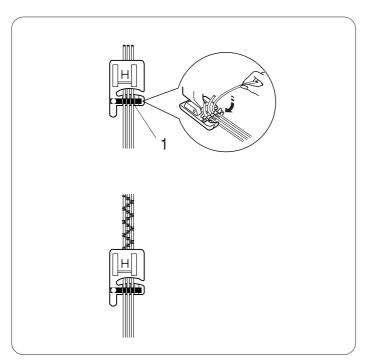
Insert 3 strands of cording under the spring of the foot and draw them under the foot to the rear.
