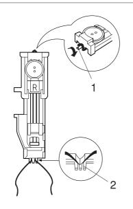
With the automatic buttonhole foot R raised, hook the filler cord on the spur at the back of the buttonhole foot
