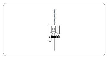
Insert one strand of cording under the spring of the foot and draw it under the foot to the rear (use the center slot of the spring).
